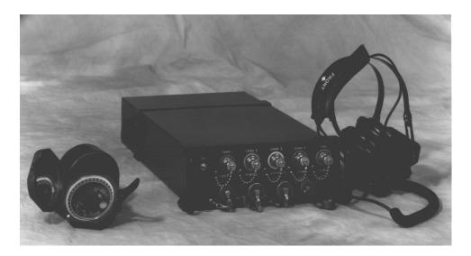
The WJ-8991 (ICE) DF system is a complete manpack Direction Finding and Intercept system based on the WJ-8996-1 Correlative Vector DF Processor. The flexibility of the ICE system allows for deployment on a variety of platforms. Available options (see table) allow customization to particular system requirements.
